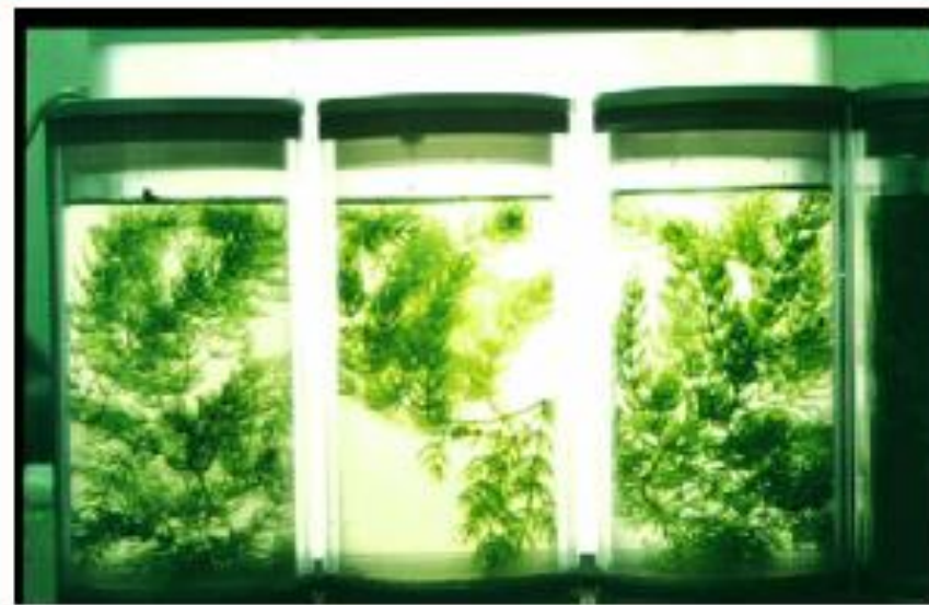
Fig.1 Returned flight ABS units (two cylindrical vessels at left) and one of the ground control units (one at right). The Space-shuttle experiment in May 1996.
