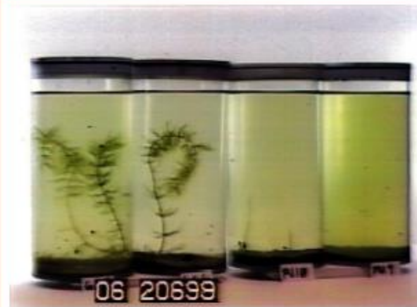
Fig.4 Ground and flight samples immediately after the first Mir experiment. Ground samples (the two cylindrical vessels at left), and the flight samples (two units at right) which were recovered after being exposed to microgravity for 4 months in Mir. Note the complete disappearance of water plant (hornwort) in the flight ABS units. The ABS unit shown here are, from left, GC8 and GC6 (the two ground units), FU10 and FU9 (the two flight units), respectively.
